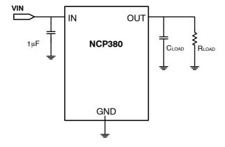
Figure 3. Test Configuration
