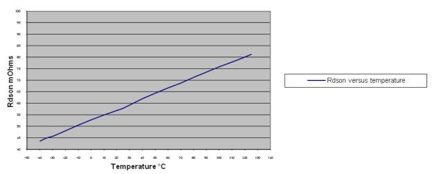
Figure 21.  $R_{DS(on)}$  vs Temperature,  $\mu DFN$  Package
