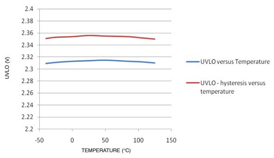
Figure 17. Undervoltage Threshold (Falling) and Hysteresis
