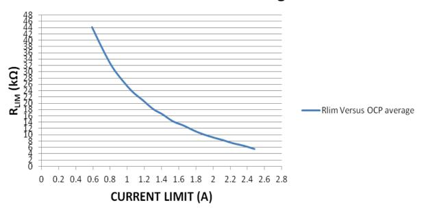
Figure 25. Rlim Curve versus Current Limit
