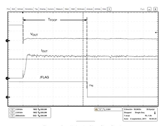
Figure 14. From No Load to Direct Short Circuit
