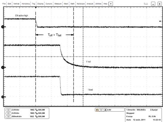
Figure 7.  $T_{\text{off}}$  Delay and  $T_{\text{fall}}$
