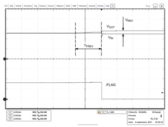
Figure 15. Reverse Voltage Detection
