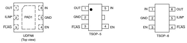
Figure 2. Pin Connections
