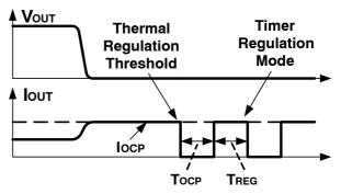
Figure 24. Short circuit
