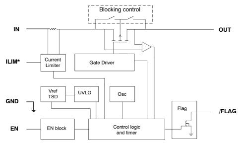
Figure 5. Block Diagram
