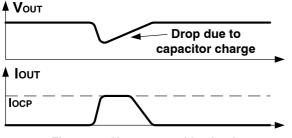
Figure 22. Heavy capacitive load
