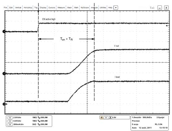
Figure 6.  $\rm T_{on}$  Delay and  $\rm T_{rise}$  Time
