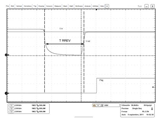
Figure 16. Reverse Voltage Removal
