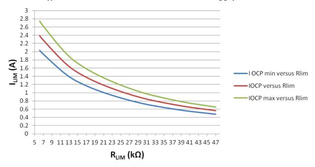
Figure 26. Current Threshold vs Rlim Resistor
