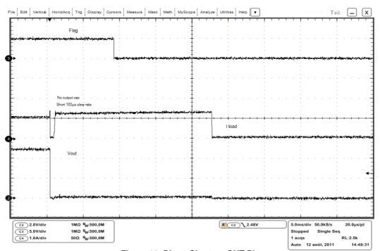
Figure 12. Direct Short on OUT Pin
