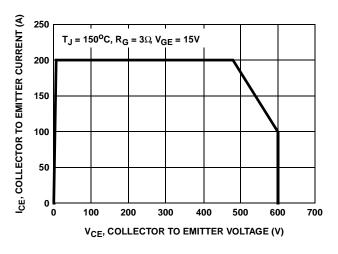
FIGURE 2. MINIMUM SWITCHING SAFE OPERATING AREA
