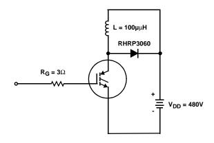
FIGURE 17. INDUCTIVE SWITCHING TEST CIRCUIT
