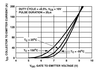
FIGURE 13. TRANSFER CHARACTERISTIC
