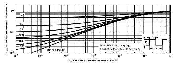
FIGURE 16. NORMALIZED TRANSIENT THERMAL RESPONSE, JUNCTION TO CASE
