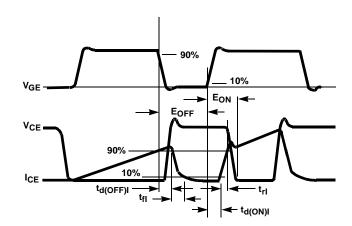
FIGURE 18. SWITCHING TEST WAVEFORM
