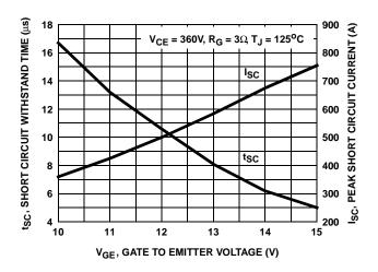
FIGURE 4. SHORT CIRCUIT WITHSTAND TIME
