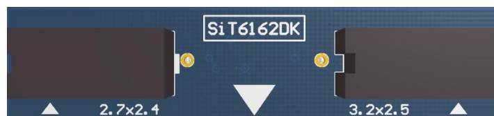
Figure 4: Time Machine socket card SiT6162DK. Supports G package (2.7mm x 2.4mm) and 3.2mm x 2.5mm packages
