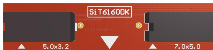
Figure 2: Time Machine socket card SiT6160DK. Supports 5.0mm x 3.2mm and 7.0mm x 5.0mm
