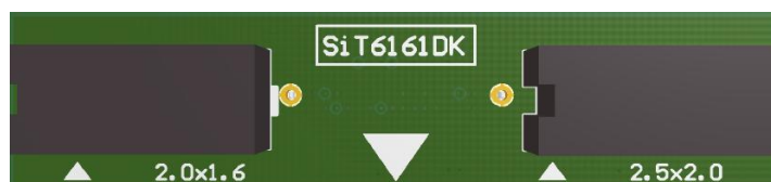
Figure 3: Time Machine socket card SiT6161DK. Supports 2.0mm x 1.6mm and 2.5mm x 2.0mm packages
