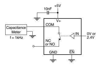
Figure 6. Channel-On Capacitance
