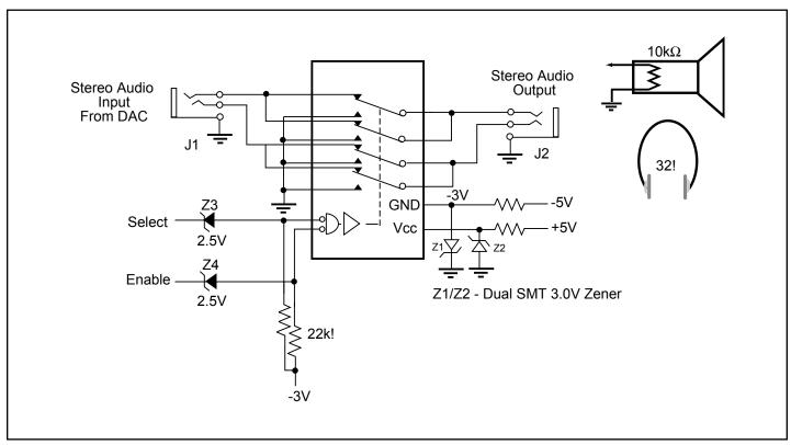
**Figure 10:** The PI5A100 momentarily mutes the stereo outputs by connecting them to ground during transition times.
