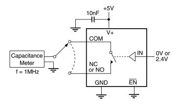
Figure 5. Channel-Off Capacitance
