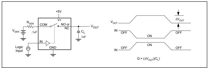
Figure 2. Charge Injection
