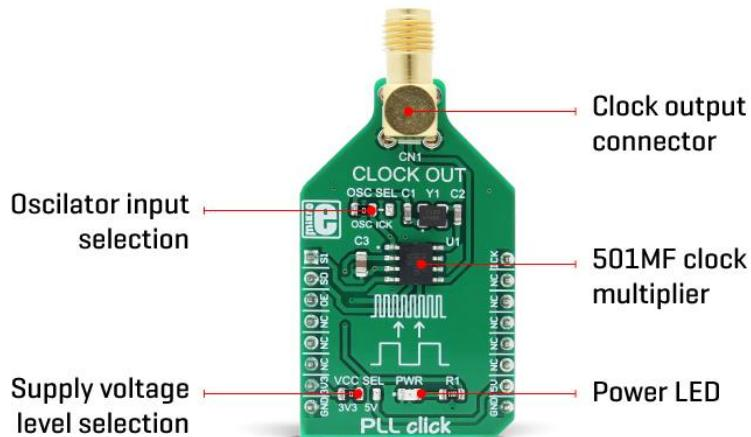
To select the desired multiplication factor, the states of the two input pins S0 and S1, routed to the mikroBUS™ pins RST and AN, respectively. These pins can be set to a HIGH logic state, LOW logic state, or can be disconnected (by tri-stating the MCU pins). The combination of these pins states will set the PLL click to a specific multiplier. To set the multiplication factor of the PLL click, please consult the multiplication selection table, below.
