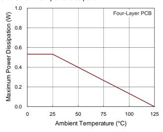
Figure 4. Derating Curve of Maximum Power Dissipation
