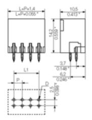
1729020000 S2L 3.5/20/180G3.5SN SW PCB plug-in connector, Male connectors, Soldered connection, Pitch: 3.50 mm, No. of poles: 20, 180°, Box 4032248040452 20 pc(s).
