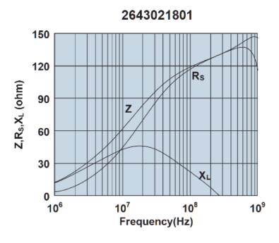
Impedance, reactance, and resistance vs. frequency.
