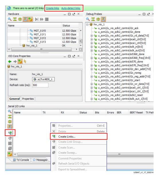
Figure 1-17: Serial I/O Analyzer - Create Links
