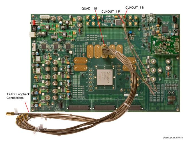
Figure 1-8: Cable Connections for Quad 115 GTX IBERT Demonstration
