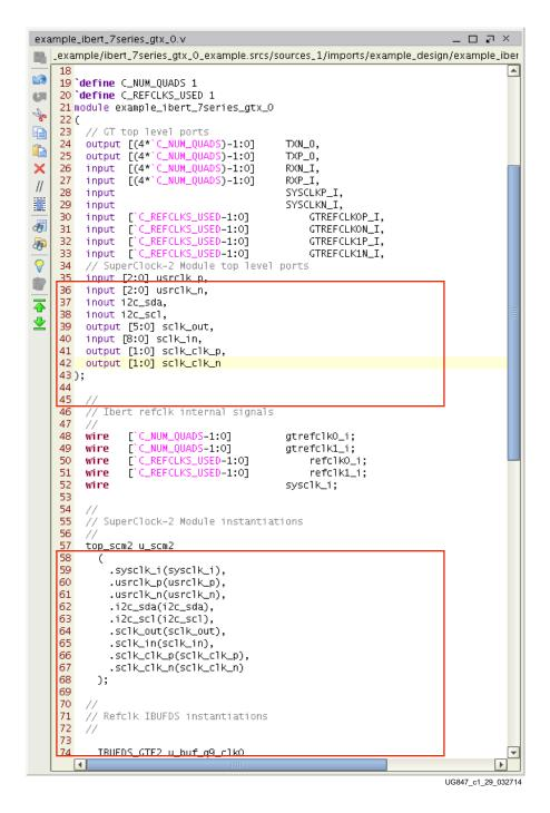
Figure 1-29: SuperClock-2 in the Example IBERT Wrapper
