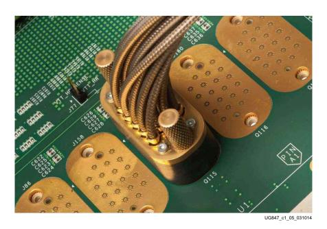
Figure 1-5: BullsEye Connector Attached to Quad 115
